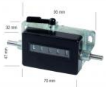
Digits height: 6 mm Both right/left drive Quick reset Max speed 5.000 rpm Zama body Weight 360 gr Strong execution suitable to be fitted on the machines
